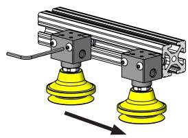
Loosen two screws, and slide the vacuum gripper to the desired location.
